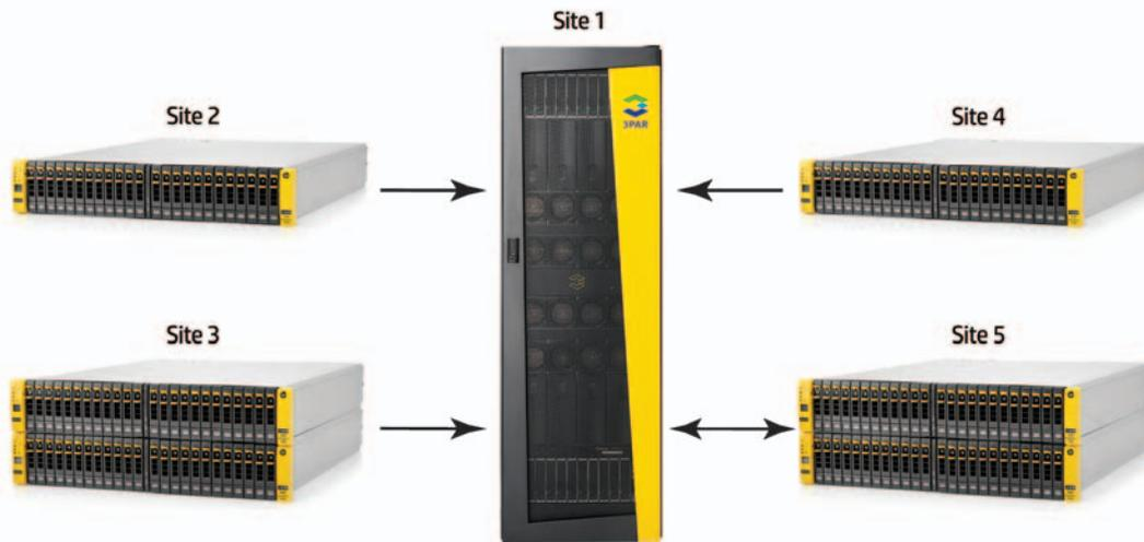
A unique suite of persistent technologies power HP 3PAR StoreServ 7000 Storage in delivering high availability and Tier 1 resiliency to the midrange. HP 3PAR Persistent Cache preserves service levels so they are not impacted by unplanned component failures—a key requirement for the virtual data center. HP 3PAR Persistent Ports allow nondisruptive upgrades to HP 3PAR StoreServ 7000 Storage systems without relying on multipathing software and without initiating failover.
