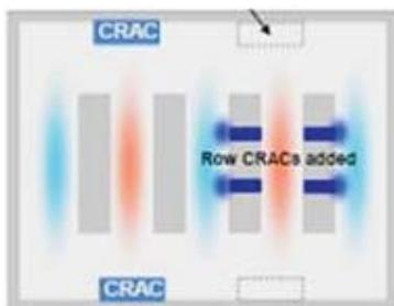
**Row based CRACs sense elevated temperature and increase fan speed to remove extra heat from hot aisle**
